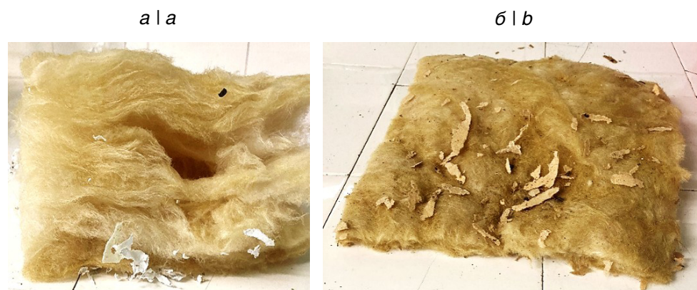
Fig. 5. Ratio of damage estimates for mineral wool and soundproofing material samples caused by brown rats when kept alone.
